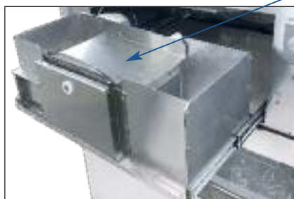
The extractable crusher unit facilitates the cleaning
