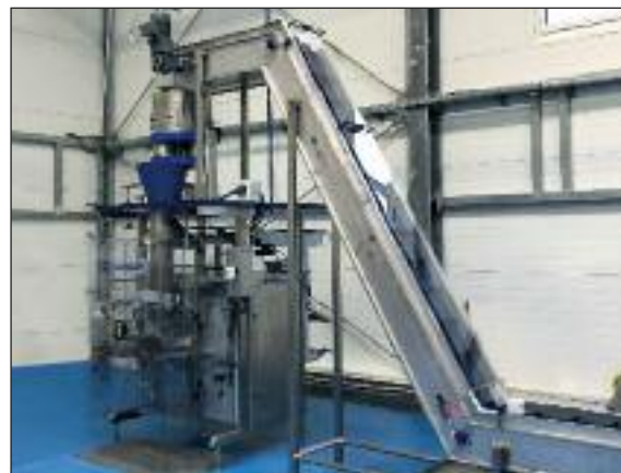
Individually designed WESSAMAT conveyor technology with automatic filling and bagging unit for ice cubes and crushed ice
