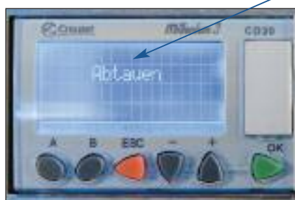
The current operating states are shown to the user via the digital display in the front panel.
