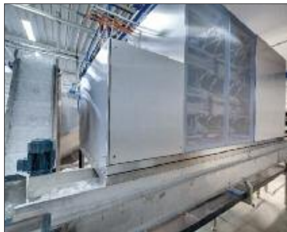
Ice preparation system IC 1500 on ice transportation belt for the production of square-sized full ice cubes
